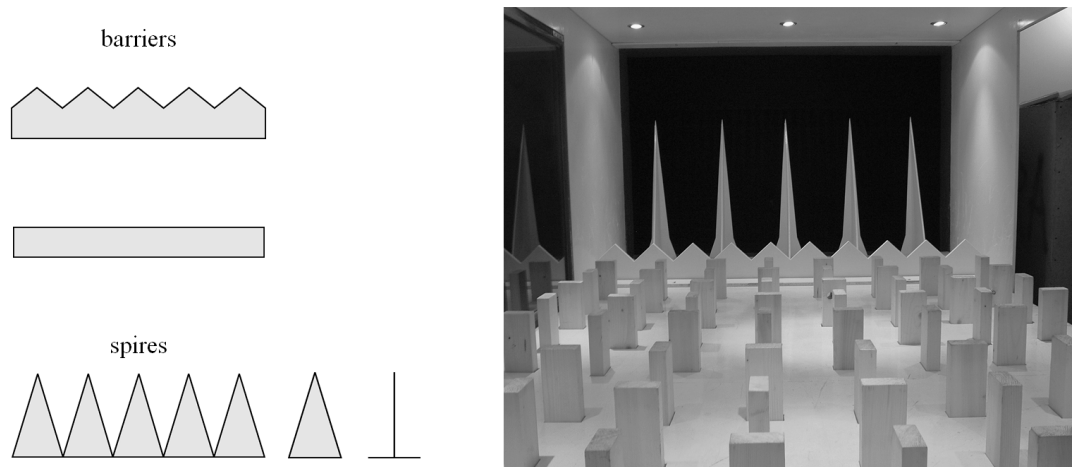
Figure 1. Turbulizers and the wind tunnel view.
