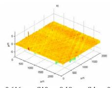
$Sq = 0.616 \ \mu\text{m}, \ S10z = 8.18 \ \mu\text{m}, \ Sdq = 0.05,$   $Spq = 0.15 \ \mu\text{m}, \ Svq = 1.52 \ \mu\text{m},$  $Smq = 94.1\%, \ Str = 0.03, \ Std = 26^{\circ}$
