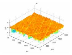
$\begin{array}{l} Sa = 0.55 \ \mu\text{m}, \ St = 7.75 \ \mu\text{m}, \ Sq = 0.87 \ \mu\text{m}, \\ Sdq = 0.089, \ Spq = 0.221 \ \mu\text{m}, \ Svq = 2.214 \ \mu\text{m}, \\ Smq = 76.3\%, \ Sp = 2.5 \ \mu\text{m}, \ Sv = 5.25 \ \mu\text{m}, \\ Ssk = -2.9, \ Sku = 13.45, \ S10z = 7.19 \ \mu\text{m}, \\ Str = 0.047, \ Std = 26^{\circ}, \ Spc = 0.01, \\ Sal = 0.022 \ \text{mm} \end{array}$
