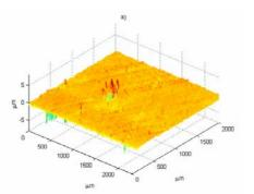
Sq = 0.49  $\mu$ m, S10z = 7.22  $\mu$ m, Sdq = 0.045, Spq = 0.14  $\mu$ m, Svq = 1.8  $\mu$ m, Smq = 94.1%, Str = 0.06, Std = 26°
