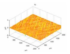
$\begin{array}{l} Sa = 0.63 \ \mu\text{m}, \ St = 6.75 \ \mu\text{m}, \ Sq = 0.89 \ \mu\text{m}, \\ Sdq = 0.088, \ Spq = 0.247 \ \mu\text{m}, \ Svq = 2.12 \ \mu\text{m}, \\ Smq = 71.6\%, \ Sp = 2.12 \ \mu\text{m}, \ Sv = 4.63 \ \mu\text{m}, \\ SSk = -2.79, \ Sku = 13.36, \ S10z = 6.57 \ \mu\text{m}, \\ Str = 0.048, \ Std = 26.5^{\circ}, \ Spc = 0.014, \\ Sal = 0.021 \ \text{mm} \end{array}$
