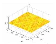
Sq = 0.62  $\mu$ m, S10z = 7.23  $\mu$ m, Sdq = 0.04, Spq = 0.12  $\mu$ m, Svq = 1.47  $\mu$ m, Smq = 90.3%, Str = 0.09, Std = 26.5°
