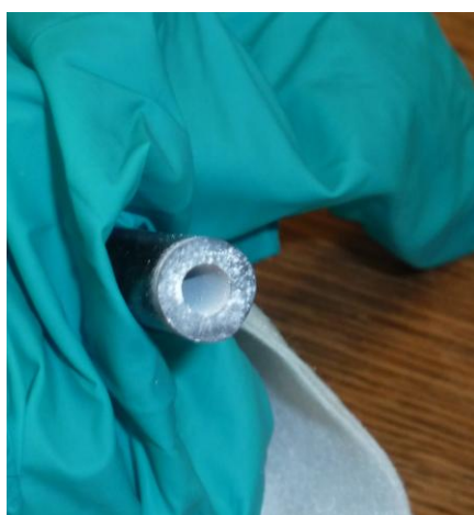
Figure 6. Picture of the SMPS sampling line inlet covered with TiO 2 powder.
