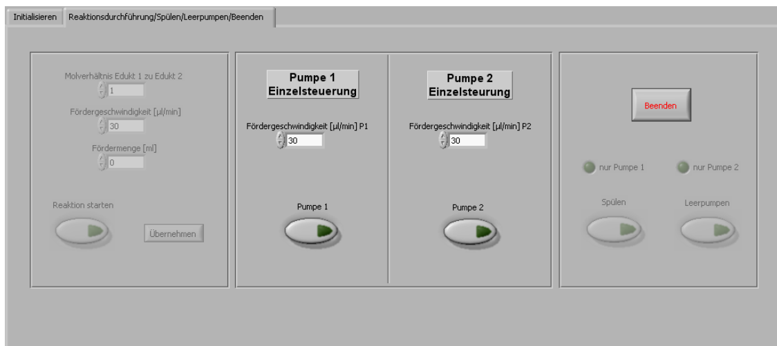
Fig. 2: Lab-VIEW 7.0 programmed „Front Panel“ for triggering the micro-pumps.
