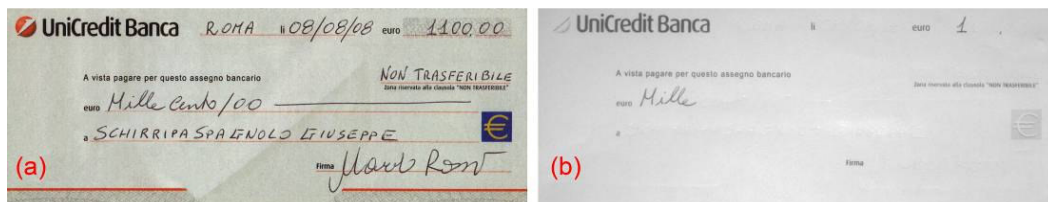
Figure 2. Example of check with fraudulent changes. Two black inks of different manufacture have been used. (a) Photo obtained using normal light. (b) Photo obtained in IR light. The difference absorption in the infrared region denote the use of two different pens.
