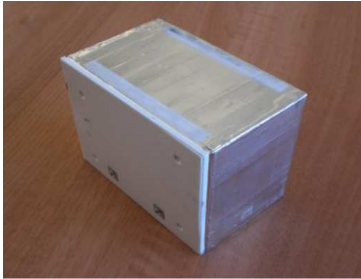
Figure 3. Emulsion Cloud Chamber brick with attached Changeable Sheet Doublet used in OPERA detector.
