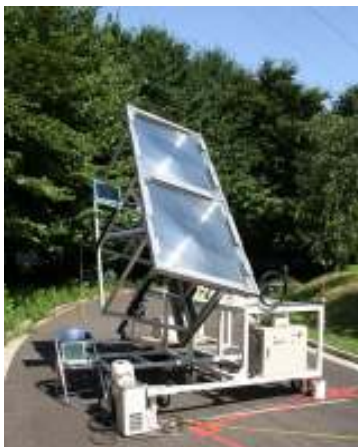
Figure1- Test system for laser from natural sunlight. Two pieces of Fresnel lens are used.
