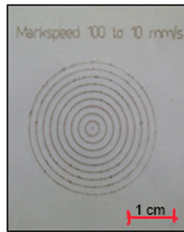
Figure 8. Circles with varying mark speed.
