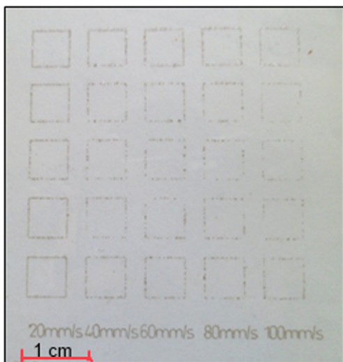
Figure 11. Power level versus mark speed.
