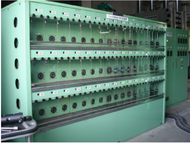
Fig. 2. Multiple-axis, cantilever-type rotating bending machine for testing gigacycle fatigue.
