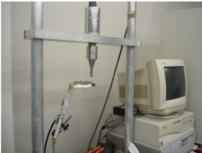
Fig. 3. Ultrasonic high-frequency machine for testing gigacycle fatigue.
