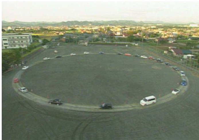
Figure 2. A snapshot of the experiment on a circular road. The circumference is 230 m, and the number of vehicles is 22. A 360-degree video camera is situated at the center of the circle for measurement.
