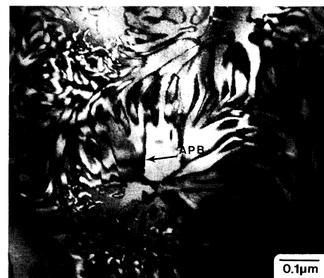
Fig. 3. Polycrystal, annealed 30 hrs. at 1000°C.
