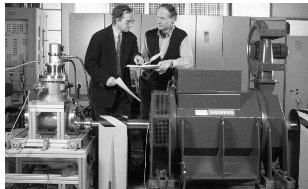
Figure 2. Photograph showing the 400 kW HTS machine in the test bed. The cooling-system with the cryocooler is located on the left side. The motor itself is mounted in a normal welded housing from a synchronous generator with a shaft height of 355 mm.
