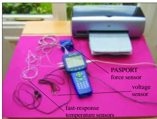
Figure 2. The Xplorer GLX , set up with an array of sensors and connected to a printer.
