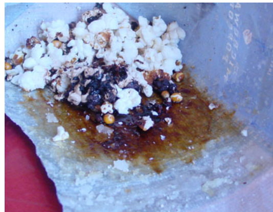
Figure 11. Top: popcorn after cooking and in its uncooked state. Bottom: the remains of the popcorn that burned on the bag—the square of aluminumized film where the temperature was greatest is clearly visible.
