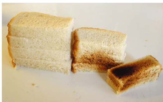
Figure 3. A section through a stack of sliced white bread before and after five minutes on full power in a microwave oven. The cooked bread is extremely hard and is noticeably smaller. The slices on the right show how the bread has blackened most inside a stack.
