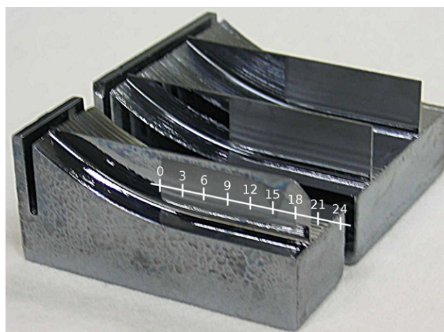
Figure 2. Photograph of the WASO 4.2a interferometer. The ruler indicates where the d_{220} measurements were carried out. The remanched area is also visible.
