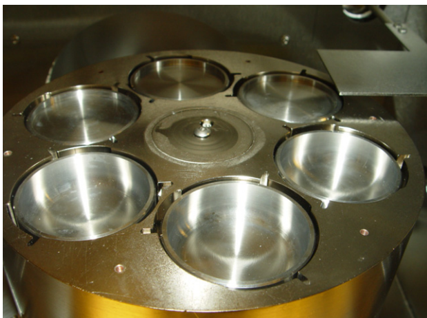
Figure 11. Photograph of a multi-target MAPLE/RIRPLD liquid nitrogen cooled stage, shown with three MAPLE cup holders for P/S mixes, and three solid target holders. Photo courtesy of PVD Products, Inc.
