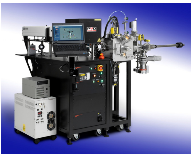
Figure 9. Photograph of a RIRPLE/MAPLE deposition system. These systems are typically set up for 50 mm diameter wafers and can handle from one to four MAPLE targets. Photo courtesy of PVD Products, Inc.
