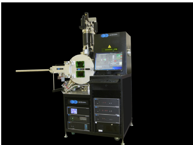
Figure 15. A photograph of a Pioneer 200 large-area PLD system to handle 200 mm diameter wafers, loadlock with substrate heating to 750 °C. Ports are provided on the chamber to add other components. Photo courtesy of Neocera, LLC.
