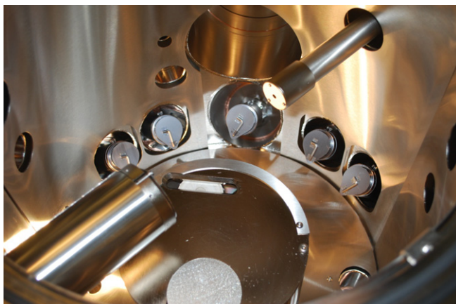
Figure 12. Photograph of the internal view of a PLD/MBE-2500 system that includes six 2 inch PLD targets (one seen through the slot in a water-cooled circular plate), five effusion cells, and a Staib high-pressure re-entrant RHEED gun and RHEED screen. Photo courtesy of PVD Products, Inc.
