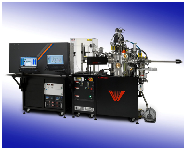
Figure 6. Photo of a commercial PLD/MBE-2300 system. The system includes a six-position 50 mm diameter target carousel, 50 mm diameter substrate holder with heating to 950^\circ\text{C} , two UHV magnetron sputter sources, HP RHEED, a dual wafer loadlock and a base pressure below 5 \times 10^{-9} Torr. Photo courtesy of PVD Products, Inc.
