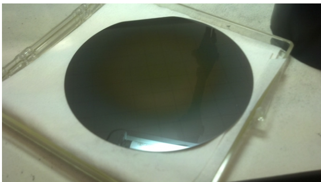
Figure 8. Photograph of a 350 kDa polystyrene film deposited onto a 100 mm diameter substrate with a RIR MAPLE technique using a system similar to that shown in figure 9. This work was conducted by the Stiff-Roberts group at Duke University.
