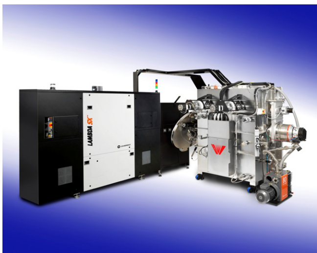
Figure 19. Photograph of a commercial reel-to-reel PLD tool capable of depositing \text{CeO}_2 or \text{LaMnO}_3 buffer layers and micrometre thick YBCO films over 1 cm wide by 1 km long Hasteloy tapes. The total effective area of such a tape is 10 \text{ m}^2 . Photo courtesy of PVD Products, Inc.
